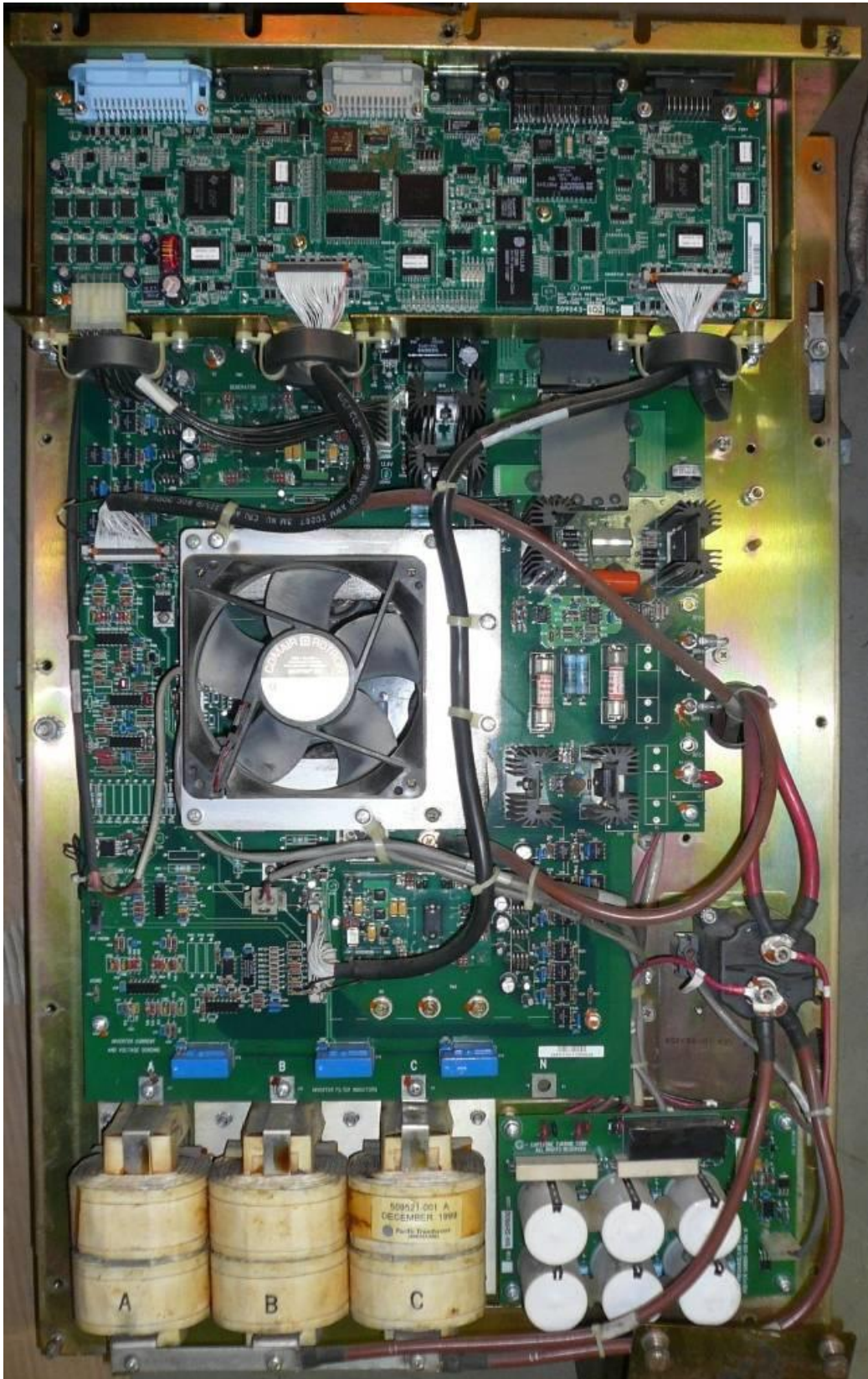
Micro-turbine control and power conditioning unit (Capstone DPC)
