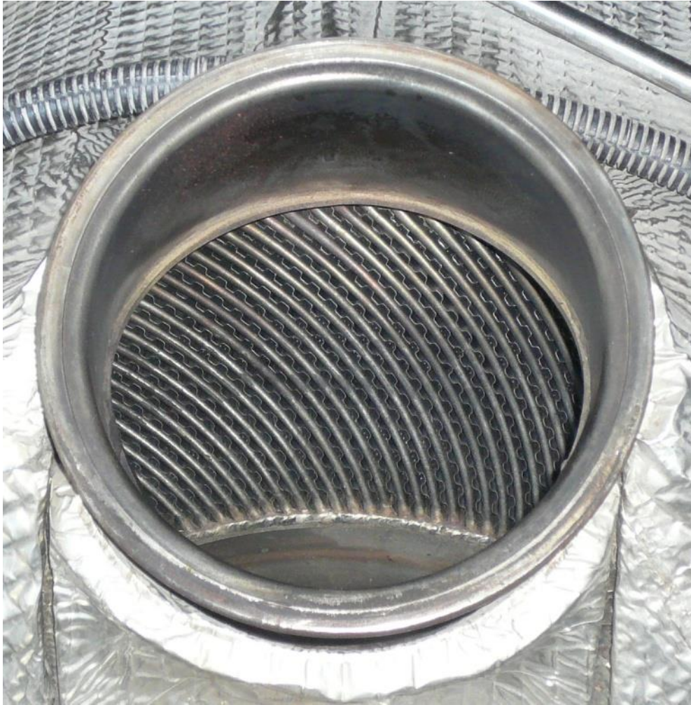
Heat exchanger exhaust outlet showing internal matrix (Capstone C30)
