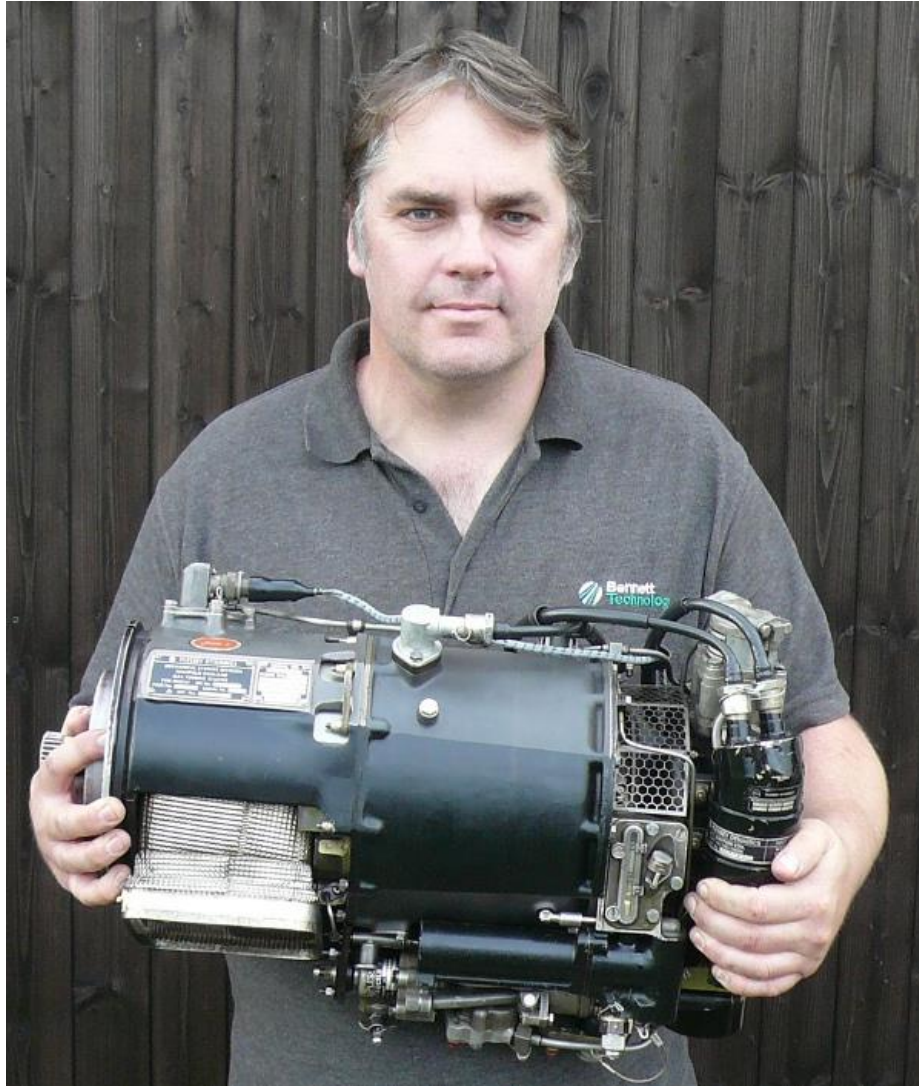
Small 70HP twin shaft gas turbine (Plessey Solent MK101)
