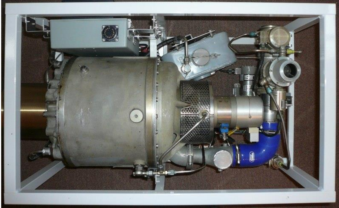
Small gas turbine featuring compressor air bleed (Microturbo)
