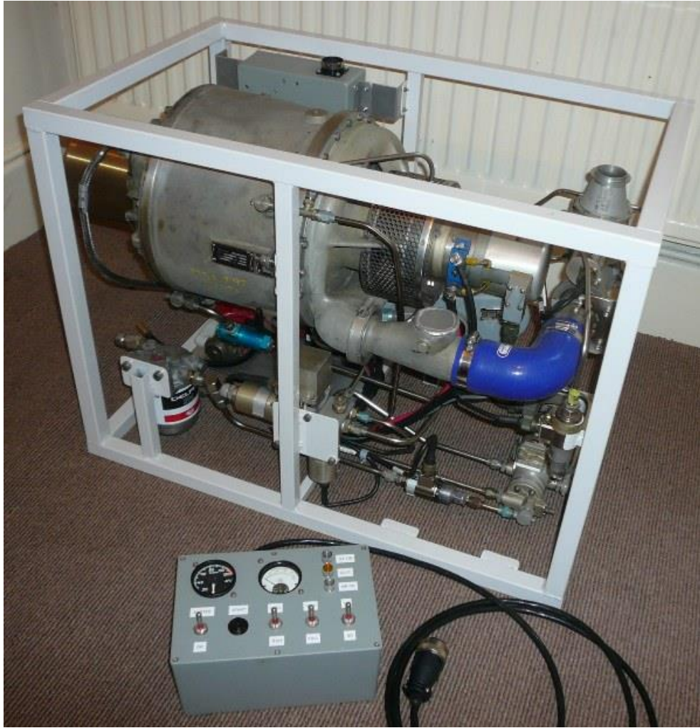
Complete assembled 50HP gas turbine engine
