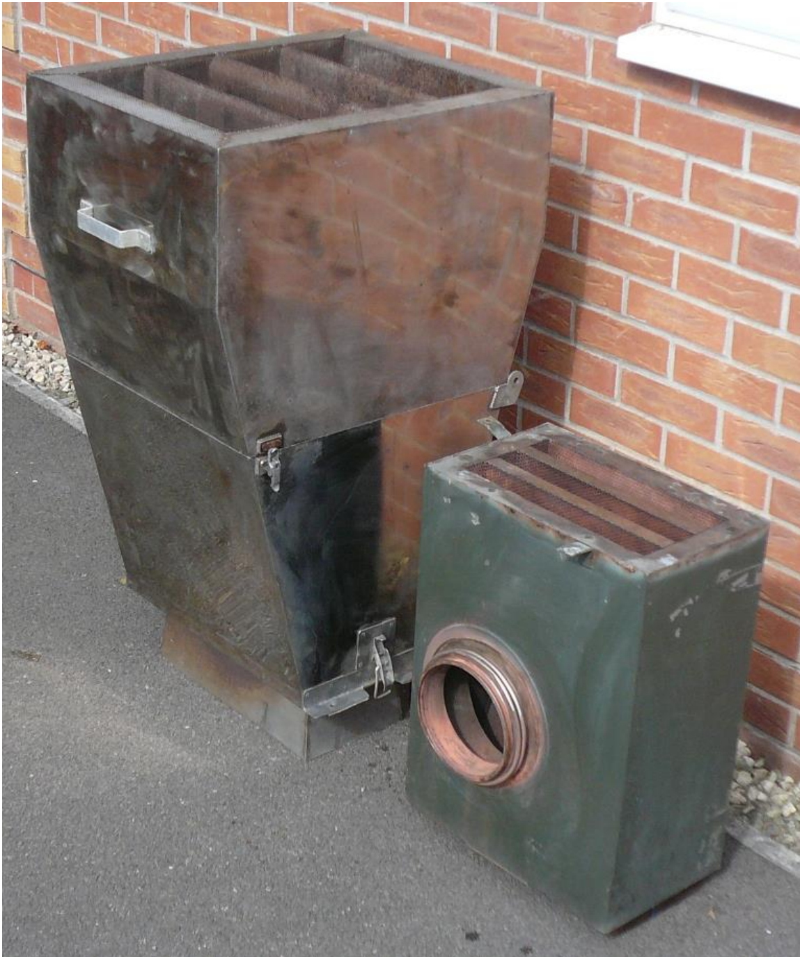
Small gas turbine exhaust silencer units (Large unit approx 1.5m high)
