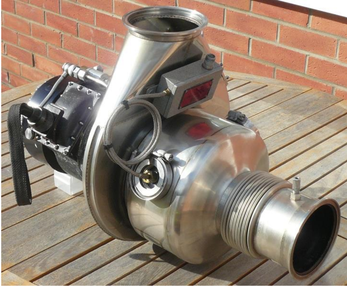
Gas turbine incorporating fluid drive coupling (Adolph Saurer GT15)
