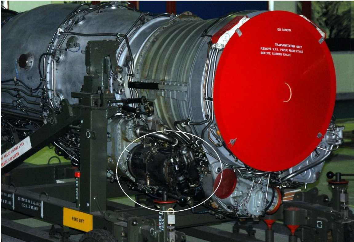
The Solent GTS MK101 fitted near the front of the RR Spey Aircraft Engine
