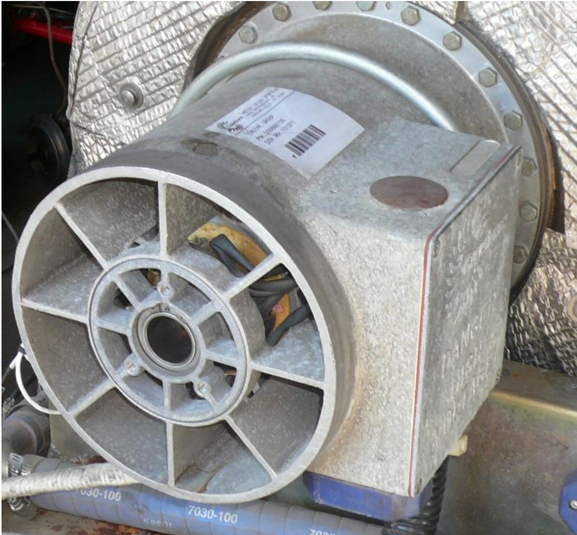
Combined micro-turbine generator unit and air intake (Capstone C30)
