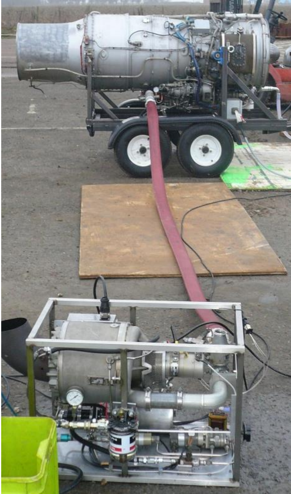
Gas turbine compressor unit used for larger engine starting
