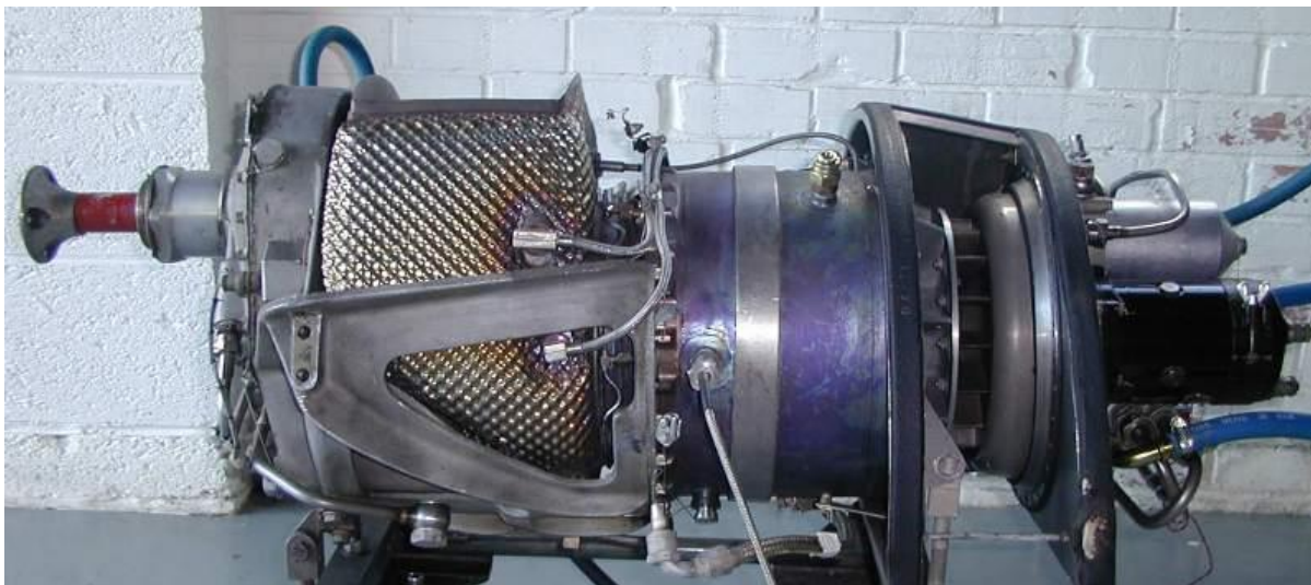
Twin shaft gas turbine engine incorporating a free power turbine stage (Rover AAPP MK10401)
